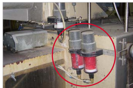
Remote pillow block lubrication on a guide pulley
