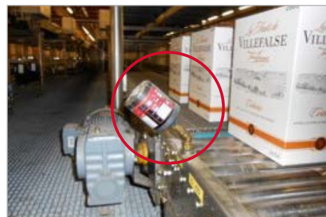
Chain lubrication of a conveyor line
