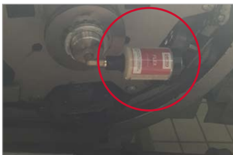
Drive pulley bearing lubrication on an oven
