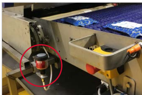
Remote flange bearing lubrication on a conveyor
