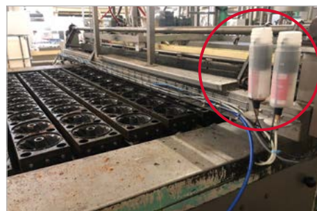
Oven chain lubrication on a baking line
