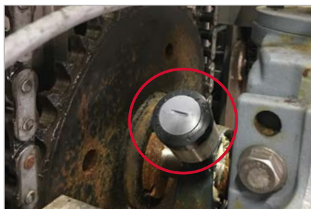
Pillow block lubrication on a drive pulley
