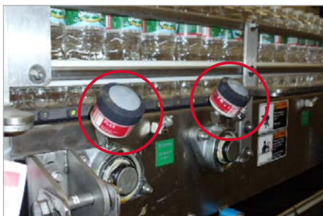
Flange bearing lubrication on a filling machine conveyor
